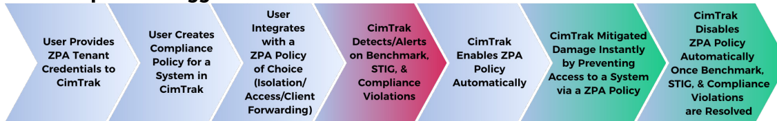
Figure 9. ZPA and CimTrak monitoring flow
